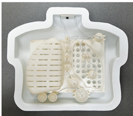
Society for Nuclear Medicine and Molecular Imaging (SNMMI) Clinical Trials Network (CTN) anthropomorphic chest phantom.
